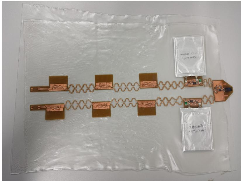
**Figure 8.6:** The demonstrator after laser-ablation and lamination
