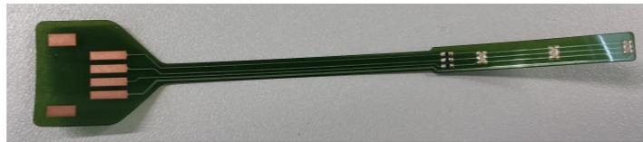
**Figure 8.5:** Single string-variant of the LED-matrix
