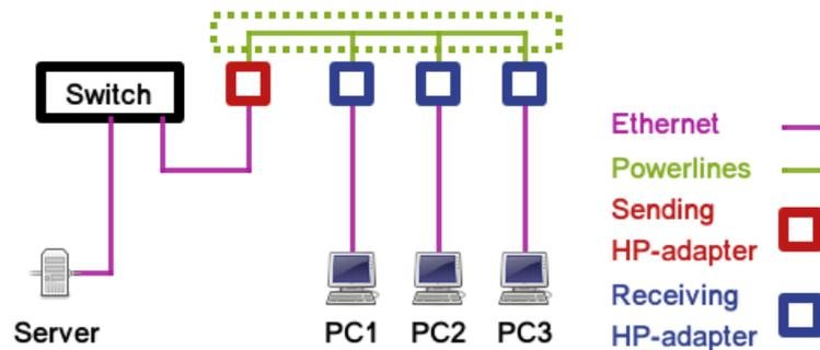
Figure 4.7: Multicast streaming – setup
