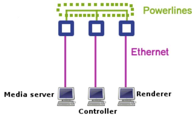
Figure 5.1: UPnP with Topcom adapters – setup
