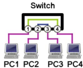
Figure 6.3: Ethernet switch
