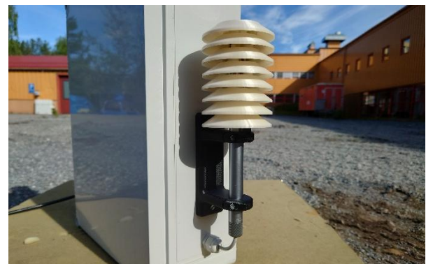
Figure 2: Temperature and humidity sensor inside the radiation shield
