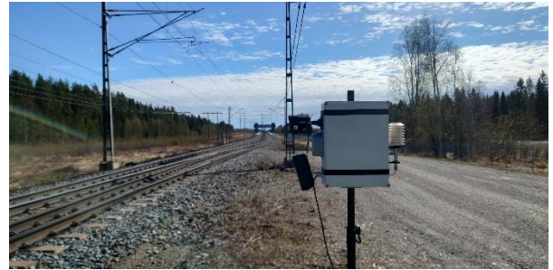
Figure 7: Measurement system near Sunderby Sjukhus station with loudspeaker as squeal simulation
