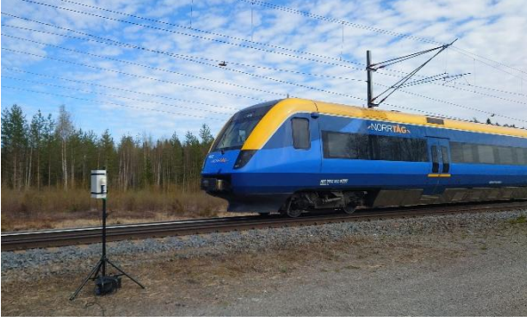
Figure 8: Measurement system during a commuter train passage
