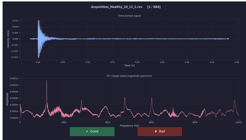
Figure 16: Manual checking of the raw vibration data was done with a Python script to make it as efficient as possible. The buttons on the bottom were used to classify them very easily. Bad measurements were deleted to ensure that they did not slip into the training data.
