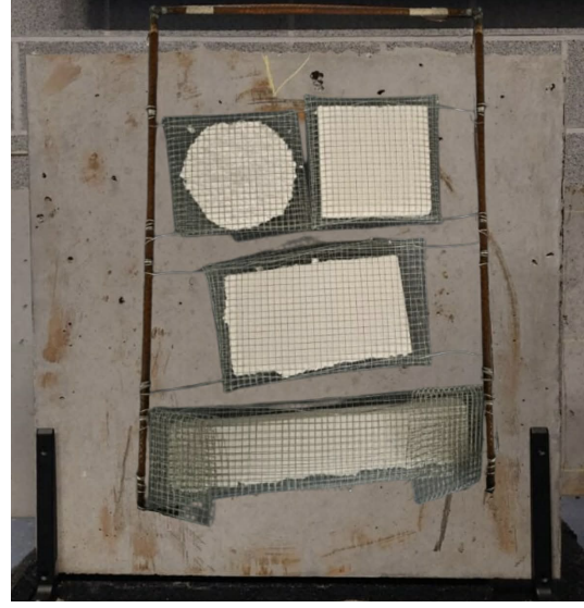
(b) Delamination block. This figure was generated using AI.
