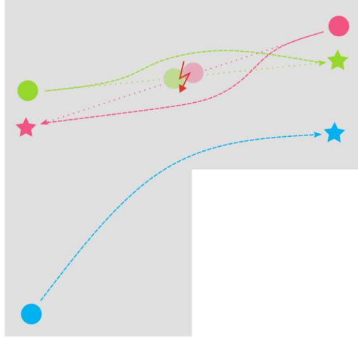
FIGURE 1.2: Multi-agent motion planning on a non-convex arena. The trajectories of the agents must be planned towards their target without collisions.
