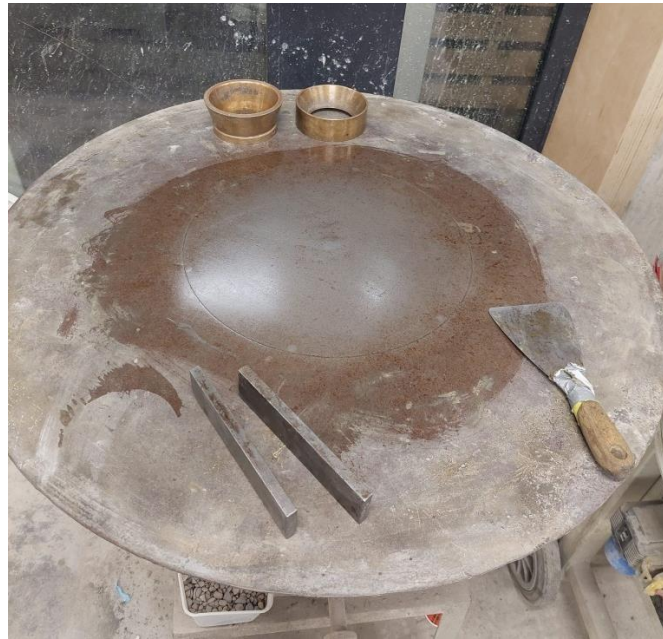
Figure 3.11: Test set-up of mini slump test
