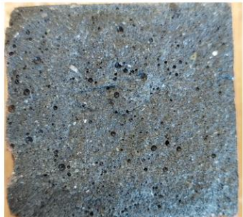
Figure 4.5: Cross section geopolymer mortars – Sea sand 0/2 mm
