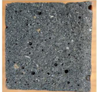
Figure 4.5: Cross section geopolymer mortars – Sea sand 0/2 mm
