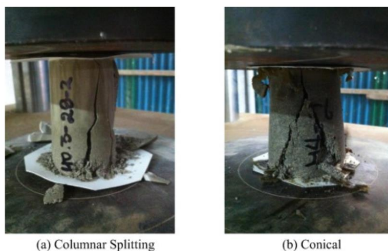
Figure 2.20: Failure modes fly ash based geopolymer mortar [71]
