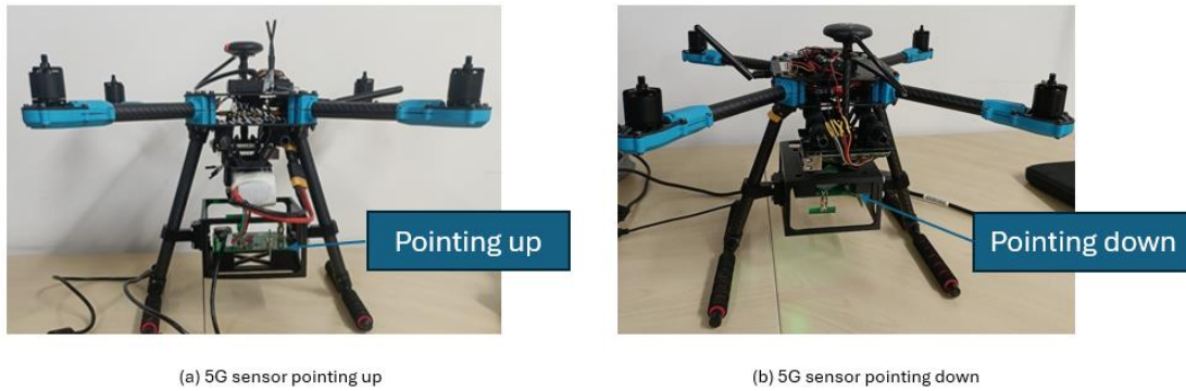
Figure 4-1: Measurement setup campaign 1: 5G sensor pointing up (a) Measurement setup campaign 2: 5G sensor pointing down (b)
