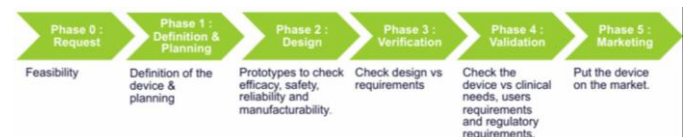
Figure 1: Medical device development cycle
