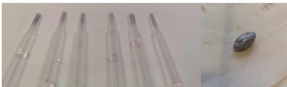
Figure 7-2: Pictures of plastic Pasteur pipets and a stirring bar, covered with gold nanoparticles after transfer and mixing of gold colloid during purification.
