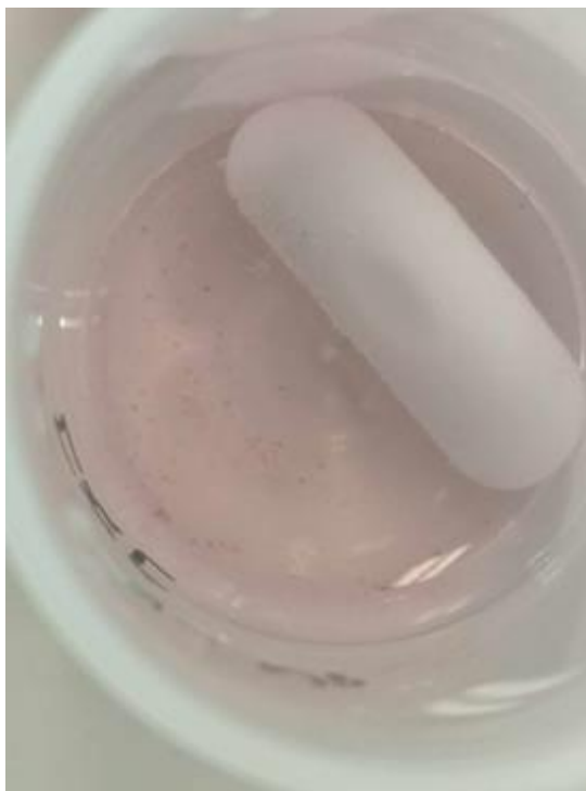
Figure 7-13: Cys-AuNP@ZIF-8 resuspended with 1 M HCl. Large visible clumps are formed, minimizing the amount of dispersed Cys-AuNPs in suspension.
