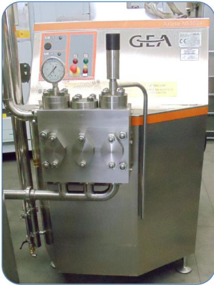
Figure 3-4: Piston pump used in Reggiani (manual)
