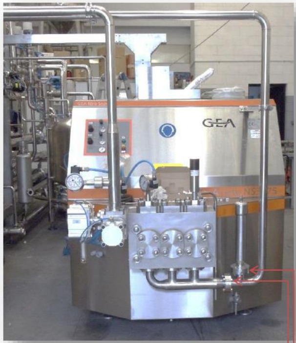
Figure 3-10: Homogenizer used in Reggiani (manual)
