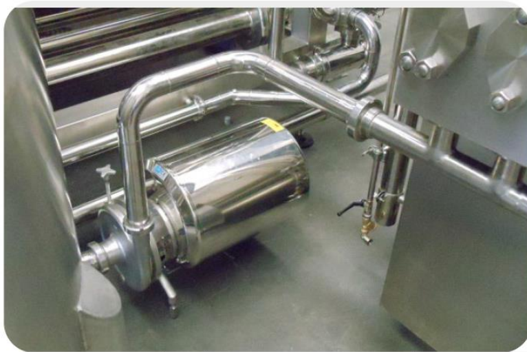
Figure 3-3: Pump PA used in Reggiani (manual)
