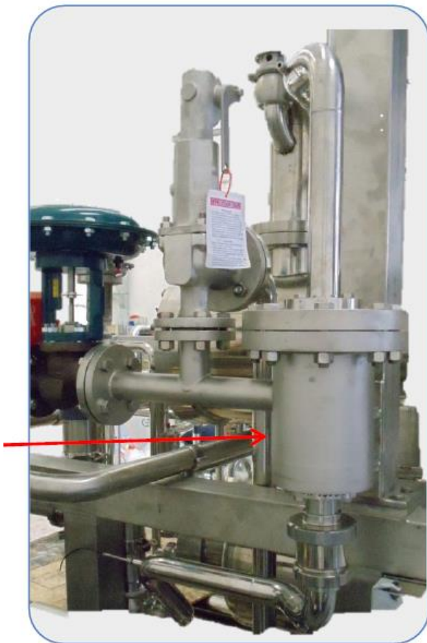
Figure 3-6: Injector used in Reggiani (manual)
