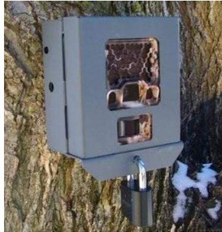
Figure 2.4: Reconyx HyperFire camera in a security box. Image from Reconyx (2013).
