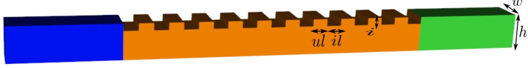
Figure 4.14: Si nanowire of width  $w = 5$  nm, height  $h = 5$  nm and 10 periodic indents of depth  $i = 1$  nm. The length of one indent is  $il = 2$  nm and the unindented length is  $ul = 2$  nm.
