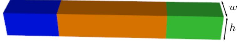
Figure 4.6: Si nanowire with a width of  $w = 5$  nm and a height of  $h = 5$  nm without a geometric superlattice.
