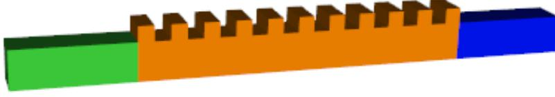
Figure 4.22: Si nanowire of 5 nm by 5 nm with fins of 2 nm height. The length of one fin is 2 nm and the spacing between the fins is 2 nm.
